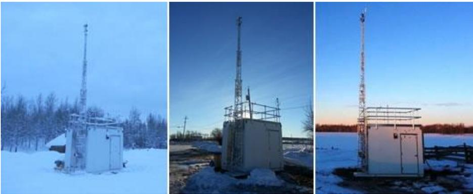
Three portable, continuous air quality monitoring stations operated at Tomslake, Doig River and Farmington in the Peace region in 2015. These stations were loaded onto a truck and transported in 2015 and 2016 to new sampling locations.
